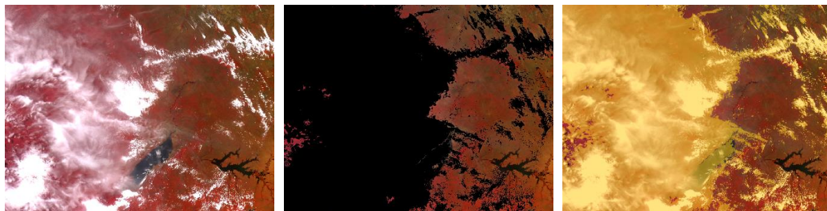
Figure 5: RGB image (left), RGB image with CLOUD mask overlay in black (middle) and in semi-transparent yellow (right) used for assessing the cloud mask
